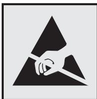
This symbol identifies static-sensitive parts. Do not touch the areas near these symbols without first touching a metal surface in an area away from the symbol.
