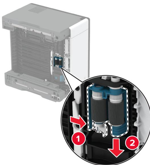
**9** Apply isopropyl alcohol to a soft, lint-free cloth, and then wipe the pick roller assembly.
