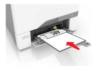
• Load envelopes with the flap side up and against the right side of the paper guide. Load European envelopes with the flap entering the printer first.
