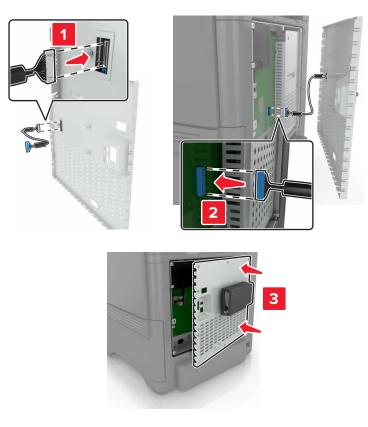
7 Reattach the controller board access cover.
