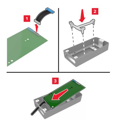
**5** Attach the housing to the controller board access cover.
