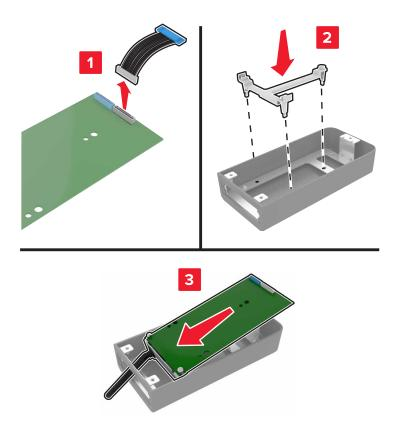
Attach the housing to the controller board access cover.
