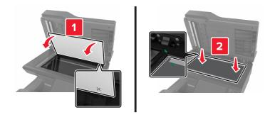
Close the scanner cover to stick the ADF scan pad to the cover.
